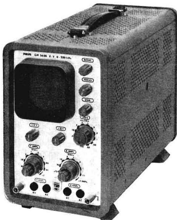
Fig. 4.18 - Oscilloscopio Philips GM 5605.
